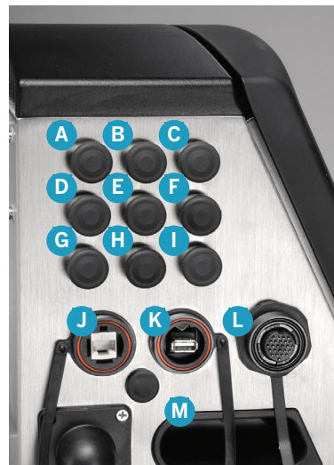
I/O ports / side panel (1620 shown)
