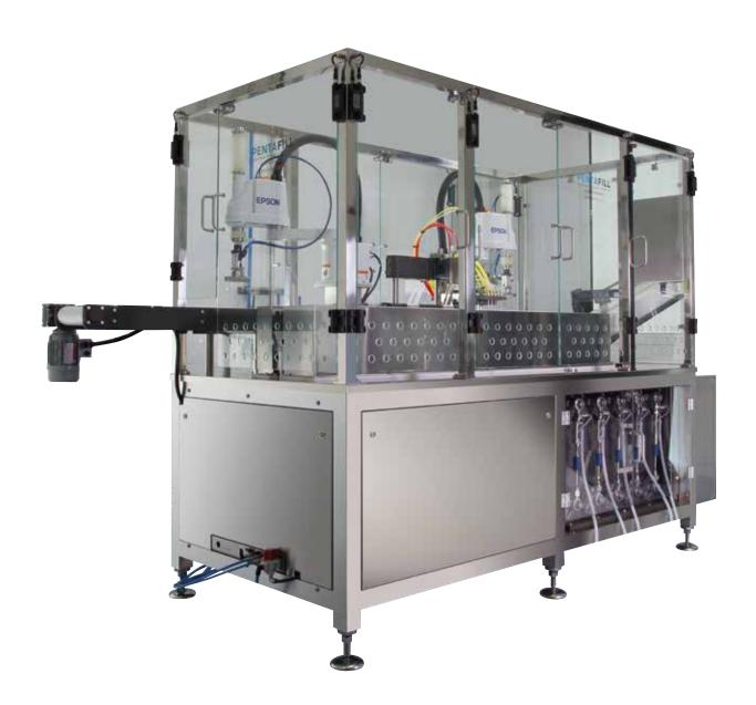
Automatic machine (25 cycles/minute) ideal for small/medium batches or start-up production.
