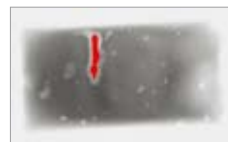
10cc air bubbles in retort foods and 2mm dia. voids in solid products are detectable.
