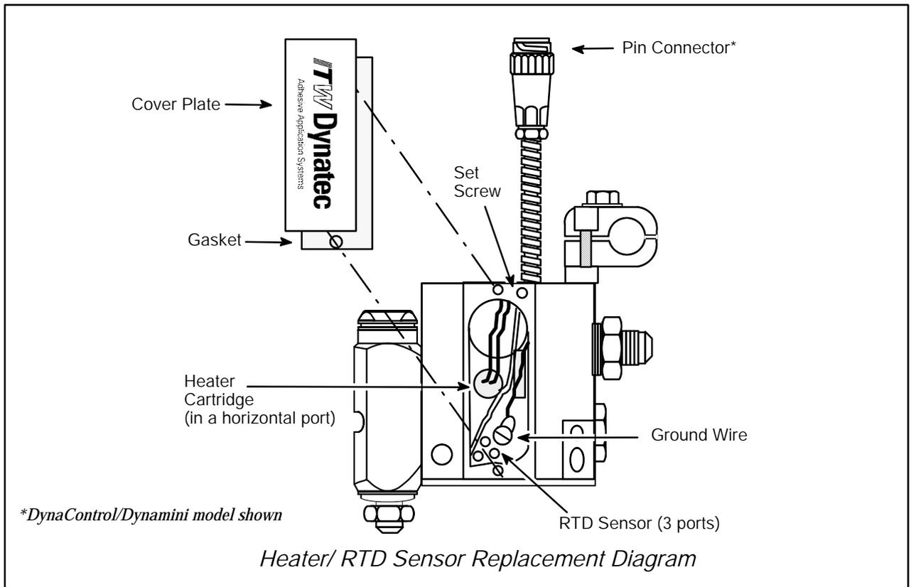
ITW Dynatec has a High Temp Heater Splice Kit available (PN 102645). Each kit contains sufficient connectors and shrink tube to replace a heater cartridge (the heater is ordered separately).
