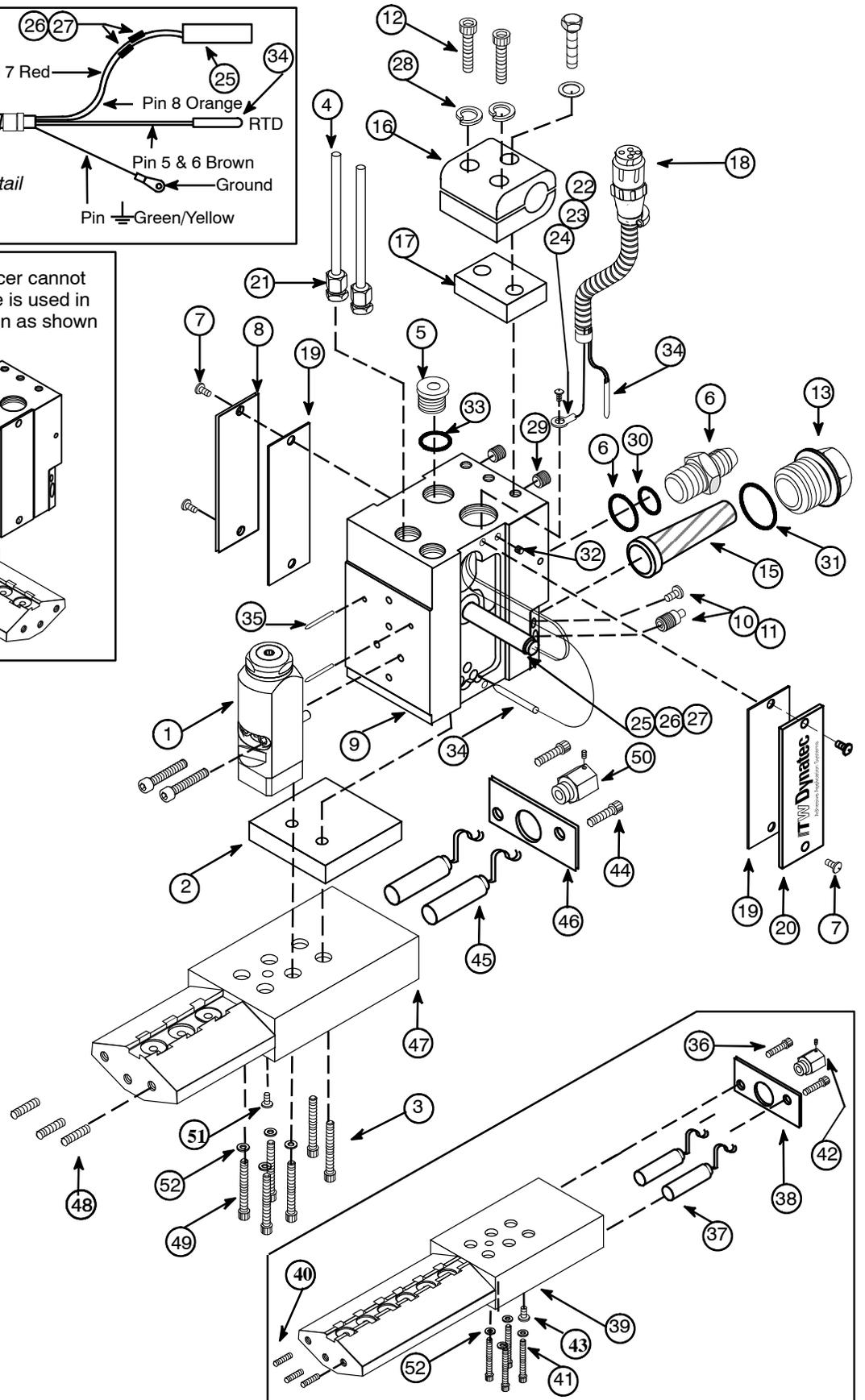
Component Illustration: Assembly 802843 & 802844 BF Head Assembly With Shoe Nozzle
