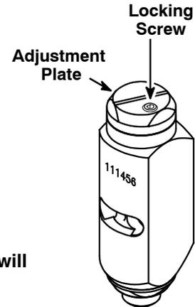
4. Back off the adjustment plate two turns (to achieve factory setting).
