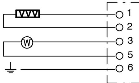
**Upgrade (SLA)** Uses PN N07958 RTD Sensor, PT100.
