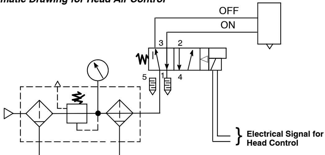
**Component Illustration: PN 100055 Air Control Filter Coalescing Kit**
