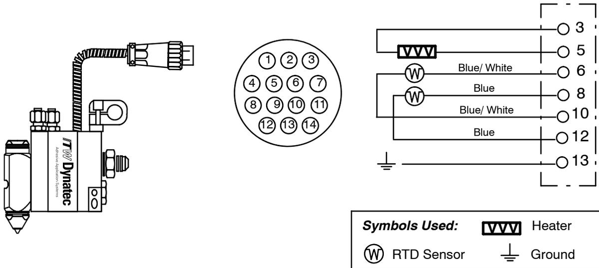
**Microprocessor Temperature Control or CompuVision (MCV)**
