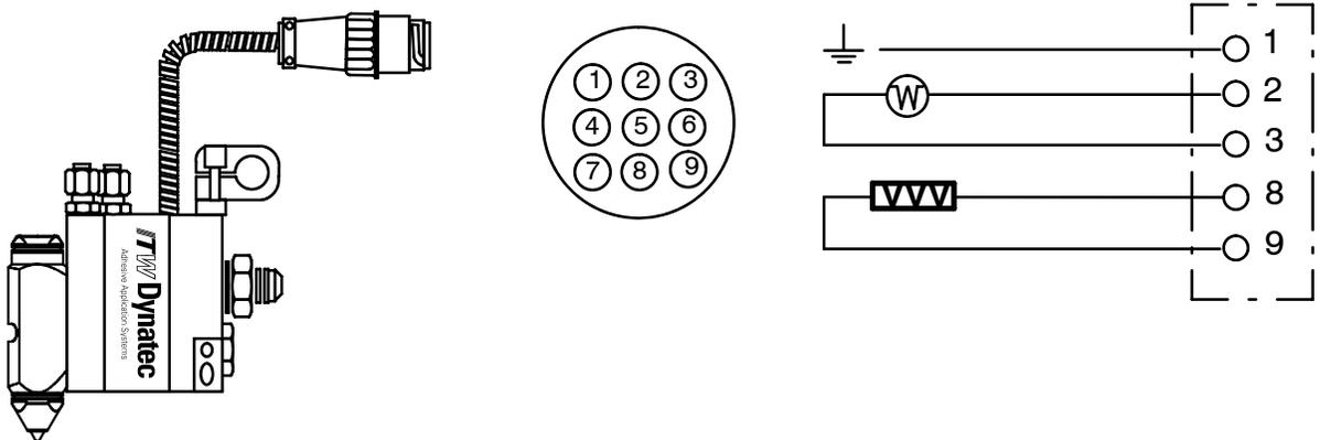
**Electronic Temperature Control with Readout (ETC)** Uses two PN N08176 RTD Sensor, NiFe.
